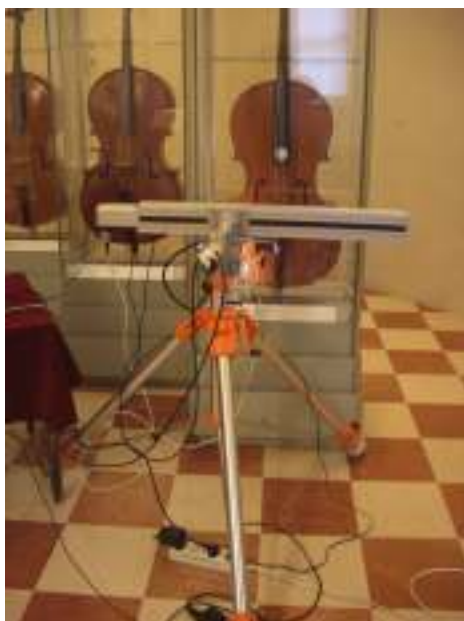
Fig. 1 - The dendrochronological measuring device used in the study. In some cases, dendrochronological analysis was possible through the instrument case.
